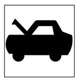
1. Pull the hood release lever with this symbol on it. It is located on the lower left side of the instrument panel.
